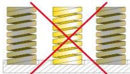
**EN** If one spring collapses, an imbalanced load will occur, possibly damaging the other springs. Replace all springs. An advance planned maintenance according to the indicated lifetime of the springs will benefit
