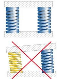
**EN** When using different type of springs in parallel simultaneously ensure that overall deflection and force guarantee a balanced load. When setting the springs ensure the best perpendicularity to the working surface to avoid early failure of the springs.
